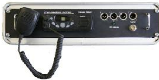
Wireless Communications for Helicopters or Remote Operators Direct RTS BP325 connection
